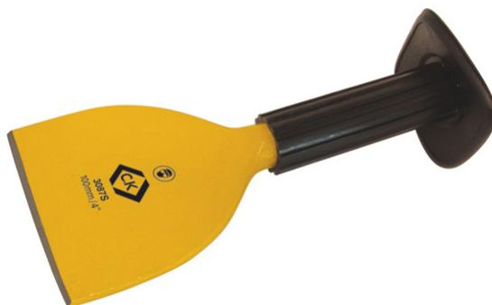
**Features & Benefits** ~ Octagonal shank brick bolster with precision ground cutting edges ~ Hardened and tempered to BS3066 for long term performance ~ Specifically designed for cutting bricks and composite blocks ~ Powder coated for corrosion protection ~ Hand guard for increased comfort and protection from overstrike ~ Length: 230 mm / 9" ~ Width: 100 mm / 4"
